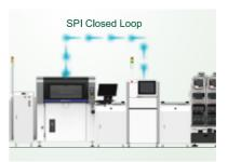
Based on inspection result feedback from SPI machines, future printing problems such as solder volume deviations, misalignment, and smearing can be predicted before they occur. Adjustment of print conditions and cleaning are performed automatically, to constantly maintain high quality printing.
