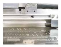
By having a load cell ready to use at the machine, printing pressure on the uneven sections of panels and masks can be controlled in real time. The optimum amount of solder filling is always achieved, even when using heavy or long squeegees with which it is difficult to fill evenly.
