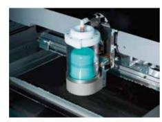
The amount of solder is detected, and solder is automatically supplied when necessary. This makes it possible to always print with the appropriate amount of solder, for stable print quality. Work can be completed without mistakes in a short time by using a solder cup as is.
