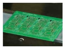
Stable clamping is achieved by using hybrid clamping, which allows users to select the optimum clamping method (side clamp/top clamp/ edge clamp) according to the characteristics of the panel.
