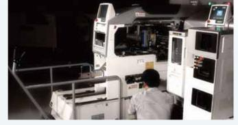
Pull the module forward and easily access the inside from both sides. Maintenance can be performed in a safe and comfortable position.
