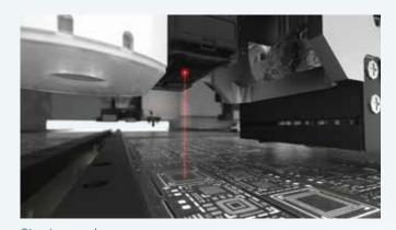
Automatically measures the panel warp by a laser sensor before placement. Production using defective panels can be prevented by using only panels within
