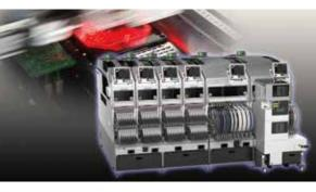
The operator just pushes the START button after exchanging the head. The machine automatically performs calibration for the head and restarts production
