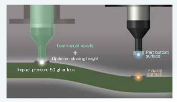
Excessive downward push and placing parts above the panel can be prevented by reflecting the part height measured by IPS to the placing surface obtained from the amount of panel warpage. Furthermore, the low impact nozzle of Fuji's original design can prevent collapse of solder and parts from being cracked.
