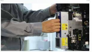
Fuji's original compact lightweight heads that can be easily exchanged withous sing tools. Operators on site can perform maintanance and handle troubles
