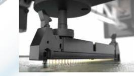
Function to push parts to reduce the manual insertion process
