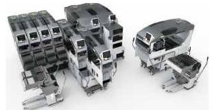
Modules, heads, and supply units can be freely exchanged based on changes in the part types and production types. This is a unique mechanism that maximizes production in the given floor space.
