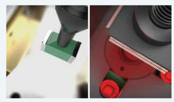
Checks for different constants, and checks for bent leads and missing bumps
