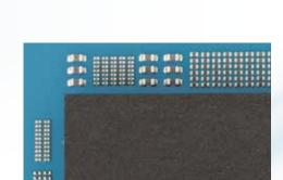
Supports high density placement for 0201 mm (008004") parts as standard Using cameras and feeders with standard specifications, 0201 (008004") parts can be placed at
