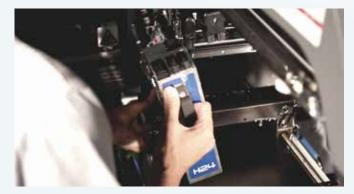
Offline maintenance maximizes the production time Exchanges units that reach the maintenance limit with units for which maintenance has been finished. Operators can easily exchange units and this can greatly reduce downtime. Perform maintenance offline on the removed units while production is still running.
