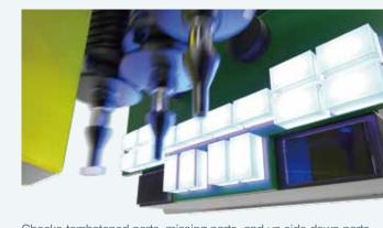
IPS can cater to a wide range of checks, from part pickup stance to parts remaining on nozzles, as well as upside-down checks for minimold parts. Placement defects caused by packaging, nozzles, and parts can be prevented.
