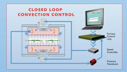
BTU's exclusive Closed Loop Convection Control provides maximum flexibility in process control.
