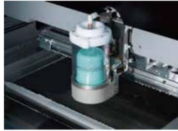
Checks solder roll diameter and automatically supplies solder when needed
