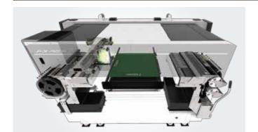
Large panel production (single robot with single conveyor)
